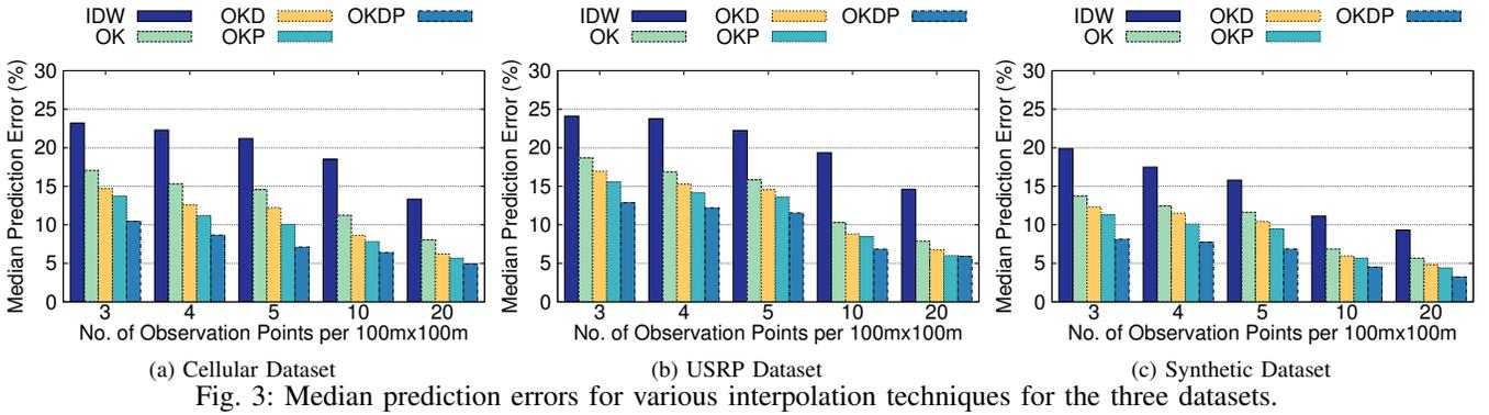
Fig. 3: Median prediction errors for various interpolation techniques for the three datasets.
