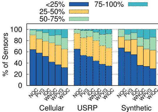
Fig. 9: Residual battery levels for various heuristics and datasets, for a fixed constraint of 4 sensors per  $100\text{m} \times 100\text{m}$ .
