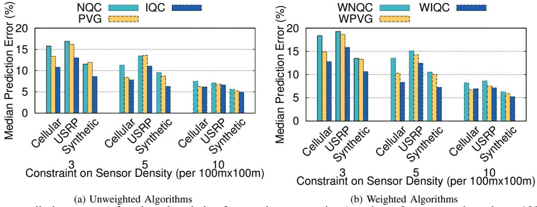
Fig. 8: Median prediction errors of various heuristics for varying constraint (number of sensors selected per  $100\text{m} \times 100\text{m}$ ), for different datasets.
