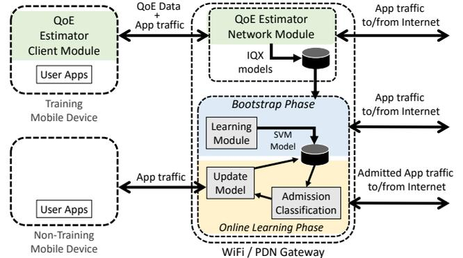
Figure 5: Software Architecture of ExBox
