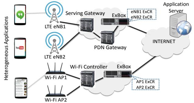
**Figure 1: ExBox is implemented as a middlebox collocated with gateway devices.**
