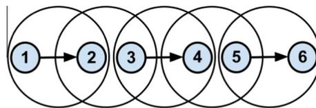
Fig. 3. An example topology to highlight imperfect channelization.
