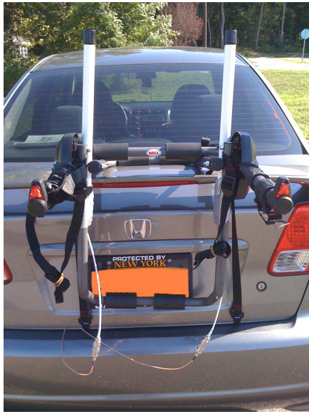
Figure 2: Two 8 dBi omni-directional antennas are mounted at the back of the car using a bicycle rack.
